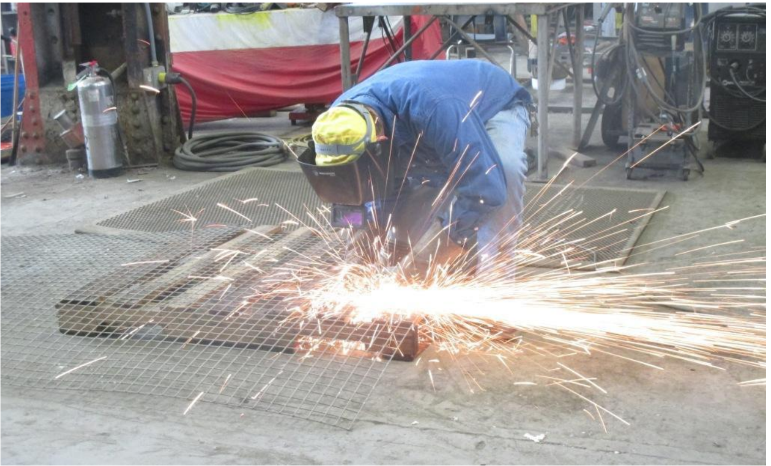
Cliff cutting metal screening to form a. engine shield for the tie-crane
