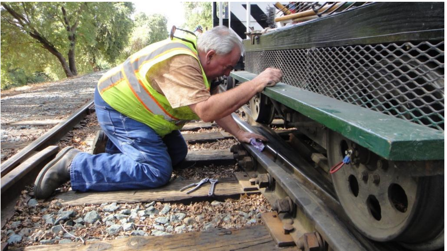
Red zone! Harry adjusts the A-6 motorcar's brakes
